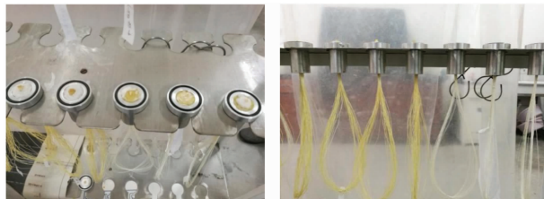
图 1 气体渗透性能测试用中空纤维膜丝标准样品 Fig. 1 Standard sample of hollow fiber membrane for gas permeability testing
