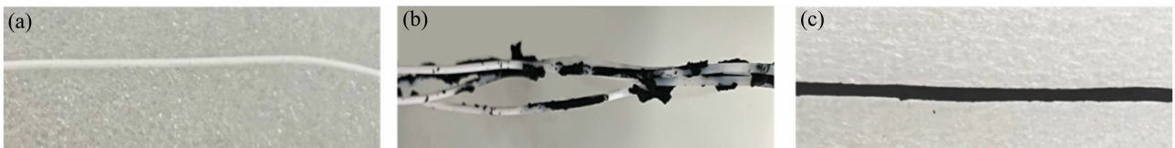
图 4 基膜 B 原膜 (a),以及用基膜 B 抽滤 m CNT 的乙醇悬浮液 30 s (b) 和 3 min (c) 后其表面外观图 Fig. 4 External surface appearance of substrate B in its original state (a), and after vacuum filtration of m CNT suspension in ethanol for 30 s (b) and 3 min (c)
